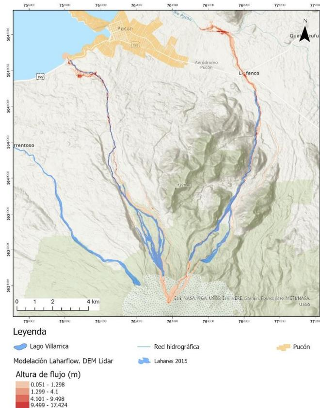
Figure 10. Lahar heights modelled for the north flank of Villarrica volcano, one the products created from high resolution DEM, used for the new detailed hazards maps for Pucón area (in yellow).
