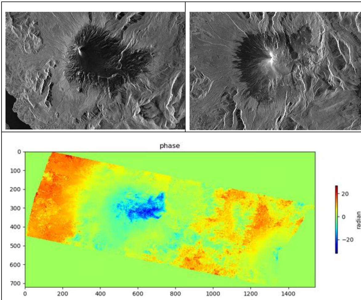
Figure 11: TerrazSARX amplitude images over Villarrica volcano in descending (left) and ascending (right) orbits. The descending image was used to create a 7 months interferogram between March 23<sup>th</sup>, 2023 and November 17<sup>th</sup> 2023, showing no deformation during this period, in agreement with GNSS data.
